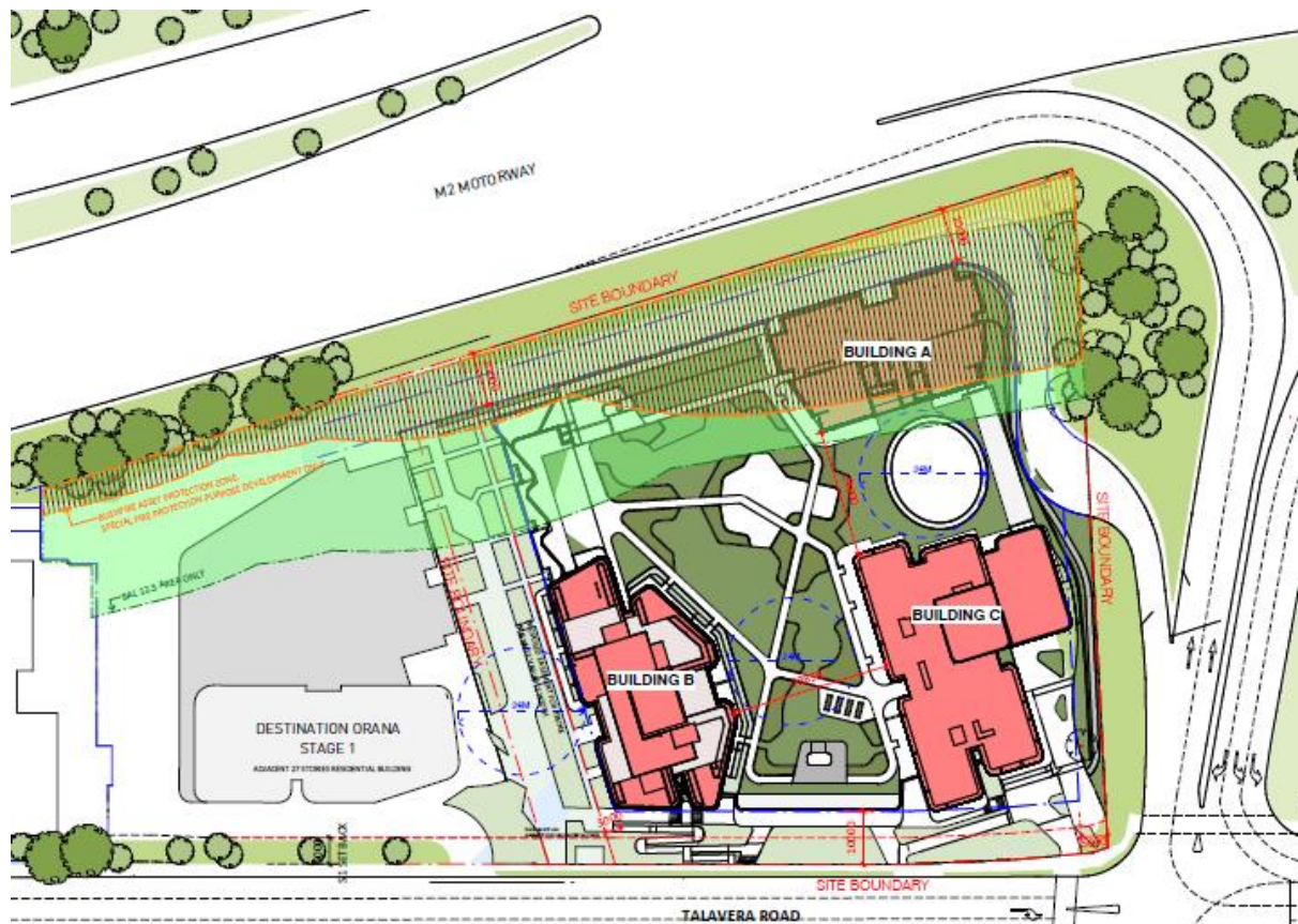
Figure 13: Site Plan showing the extent of the site orientated towards Lane Cove National Park (top) which is mapped as Bushfire Attack Level (BAL) 12.5 (green) and Bushfire Asset Protection Zone (orange).
